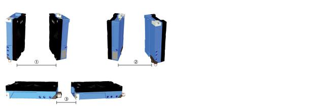
Distances required to prevent mutual interference with mounting of two devices.
