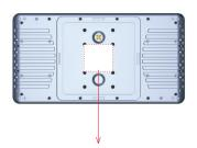
Install the antenna on the 3D mounting kit 52010351, using four M6 threaded bolts at intervals of 100 x 100 mm.
