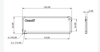
Measurements shown in mm
