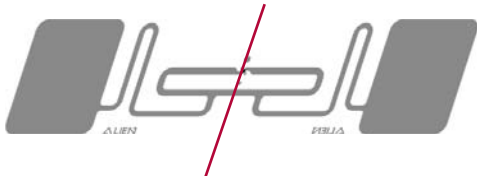
Angular Sensitivity Inlay is rotated in the x, y, plane about the z axis
